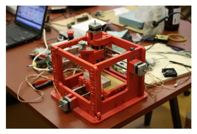
Jonathan Ward from the MIT Center for Bits and Atoms has designed a snaptogether, desktop-sized CNC milling machine. The MTM Snap (part of the Machines that Make project) is made from 12 mm high-density polyethylene (HDPE) - itself milled on a CNC- and can be assembled for about \$200. This three-axis CNC machine can mill circuit boards, wax molds, and harder materials in a 127 x 76,2 x 44,5 mm working area. Perfect demonstration project!
